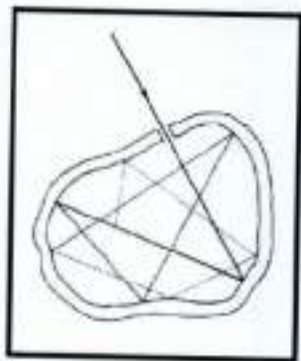
Figure 1. Incident radiation is completely adsorbed after successive reflections. The radiation emitted by the hole will have a blackbody spectrum
